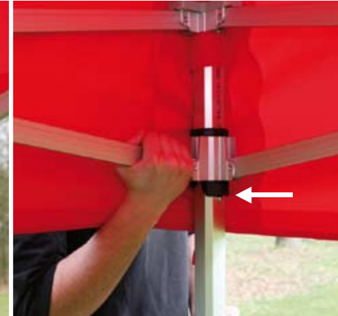
STEP 6 THE CORRECT POSITION HAS BEEN REACHED WHEN THE SLIDER CLICKS OVER THE LOCK PIN
